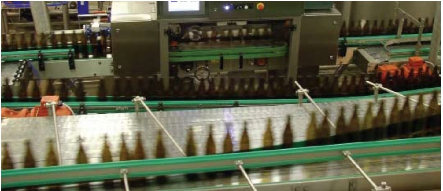
Bottling line equipped with bottle inspection system
