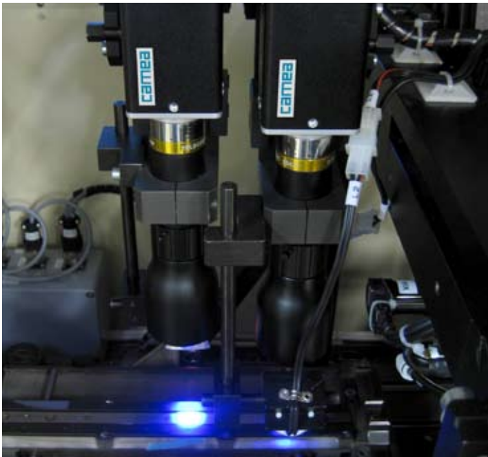
Positioning measurement taken with cameras and stroboscopic illumination system
