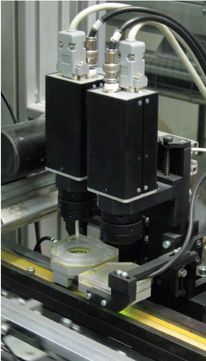
Visual surface defects inspection on a production line
