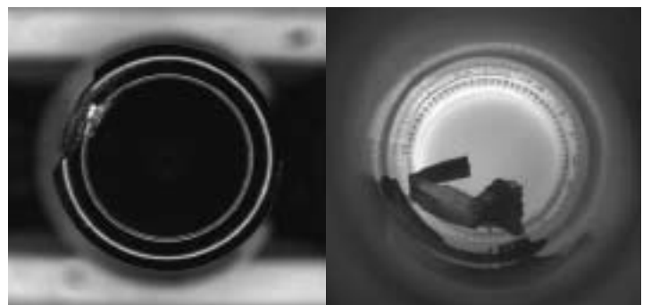
Detected defects on a bottle neck (left) and inside a bottle (right)
