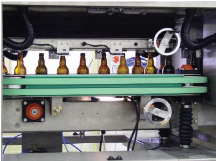
BTCAM612 visual inspection system applied in industry
